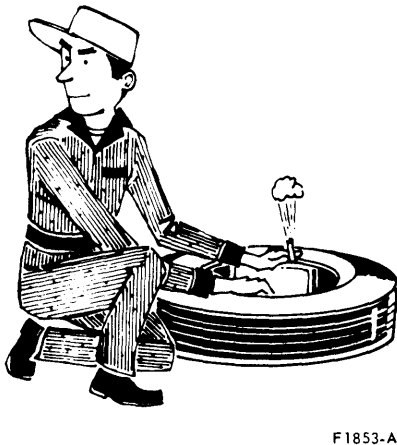
FIG. 2 Safe Air Removal
