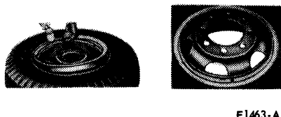
FIG. 4 Starting Locking Ring and Locking Ring Installed—Three-Piece Rim
