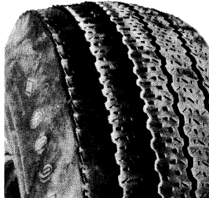
FEATHERING DUE TO MISALIGNMENT OR SEVERE CORNERING
