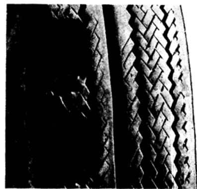
CUPPING—UNDERINFLATION AND/OR MECHANICAL IRREGULARITIES
